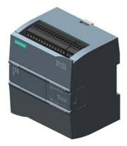
SIMATIC S7-1200, CPU 1211C, compact CPU, DC/DC/DC, onboard I/O: 6 DI 24 V DC; 4 DO 24 V DC; 2 AI 0-10 V DC, Power supply: DC 20.4-28.8V DC, Program/data memory 30 KB
